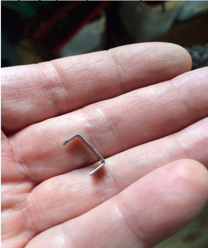
Just straighten out one leg, then push the straight end into the green and blue sides of the connector block.
